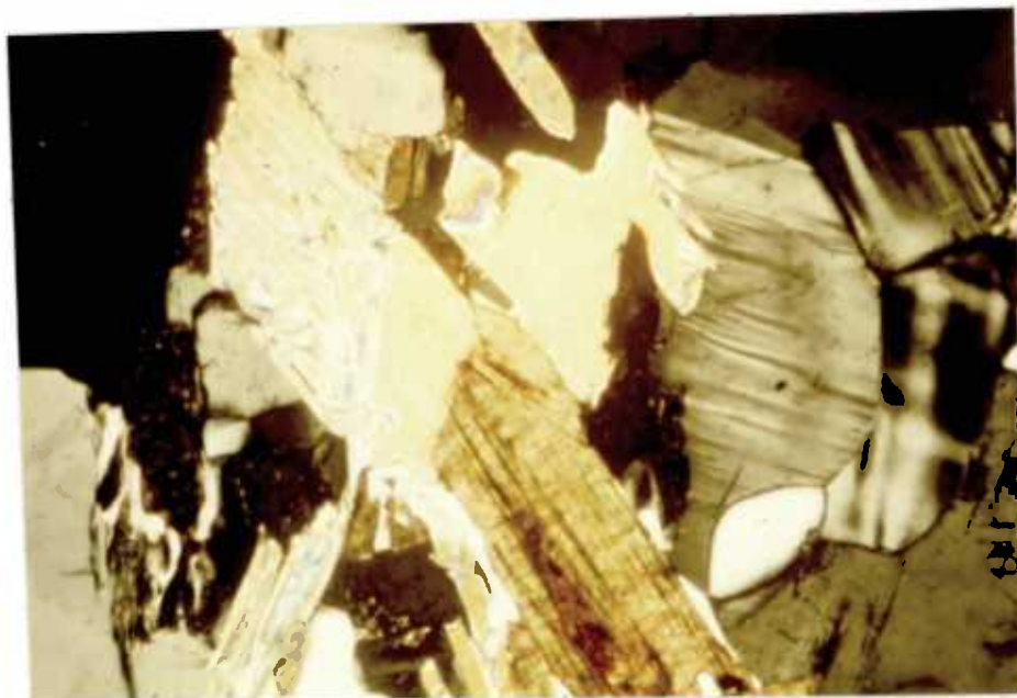
Plate 3.1. Biotite replacing potash feldspar in quartz feldspathic gneiss, Foindle. Slide No. 51610. x 160. Crossed Nicols.
