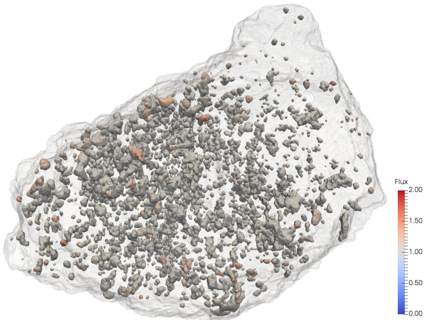
Figure 4.33: Grain-type voxels that are completely leached are replaced by gangue-type voxels increasing the particle's permeability over the simulation time. a) Initial condition b) Mid simulation time with fluxes rendered on the grains' surface.
