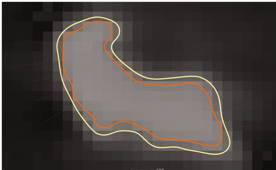
Figure 2.11: Partial volume effect, the boundary between the bright phase (grain) and the gangue gets blurred making hard to distinguish the actual location of the transition between the different minerals. From Le Roux et al. (2015).
