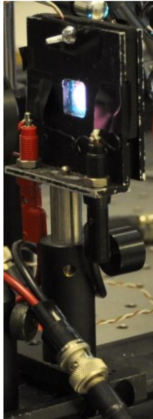
Figure 9-6 – Homemade Cell holder for the Simultaneous TA TE setup.
