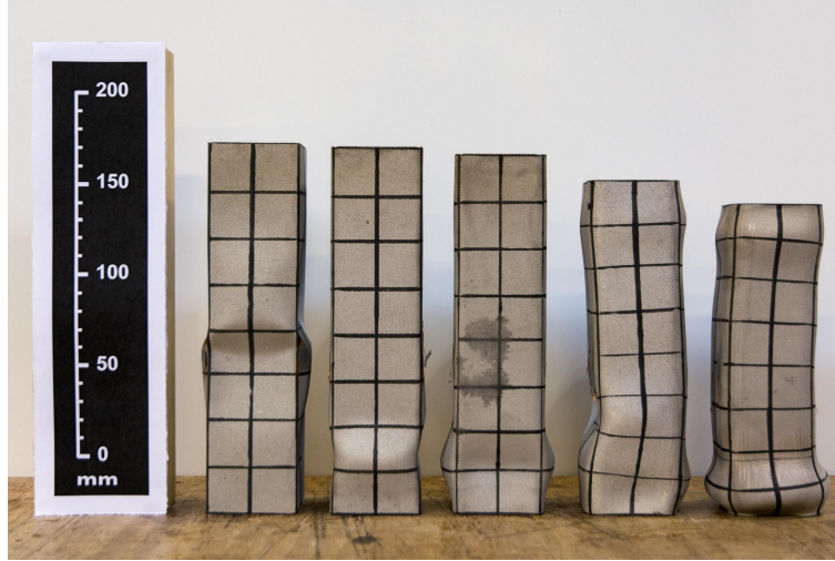
Figure 24: Deformed SHS stub columns, with increasing wall thickness from left to right
