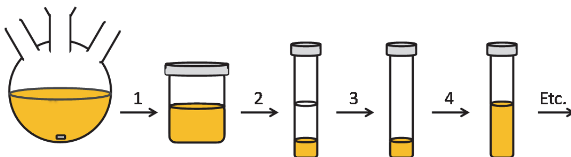
Figure 2.2. Schematic of washing procedure. 1. Quench reaction in room temperature toluene, 2. Precipitate QDs by addition of methanol, centrifuge to separate, 3. Decant colourless solution, 4. Re-disperse QDs in toluene. Repeat steps 2-4 for every subsequent washing “cycle” twice.
