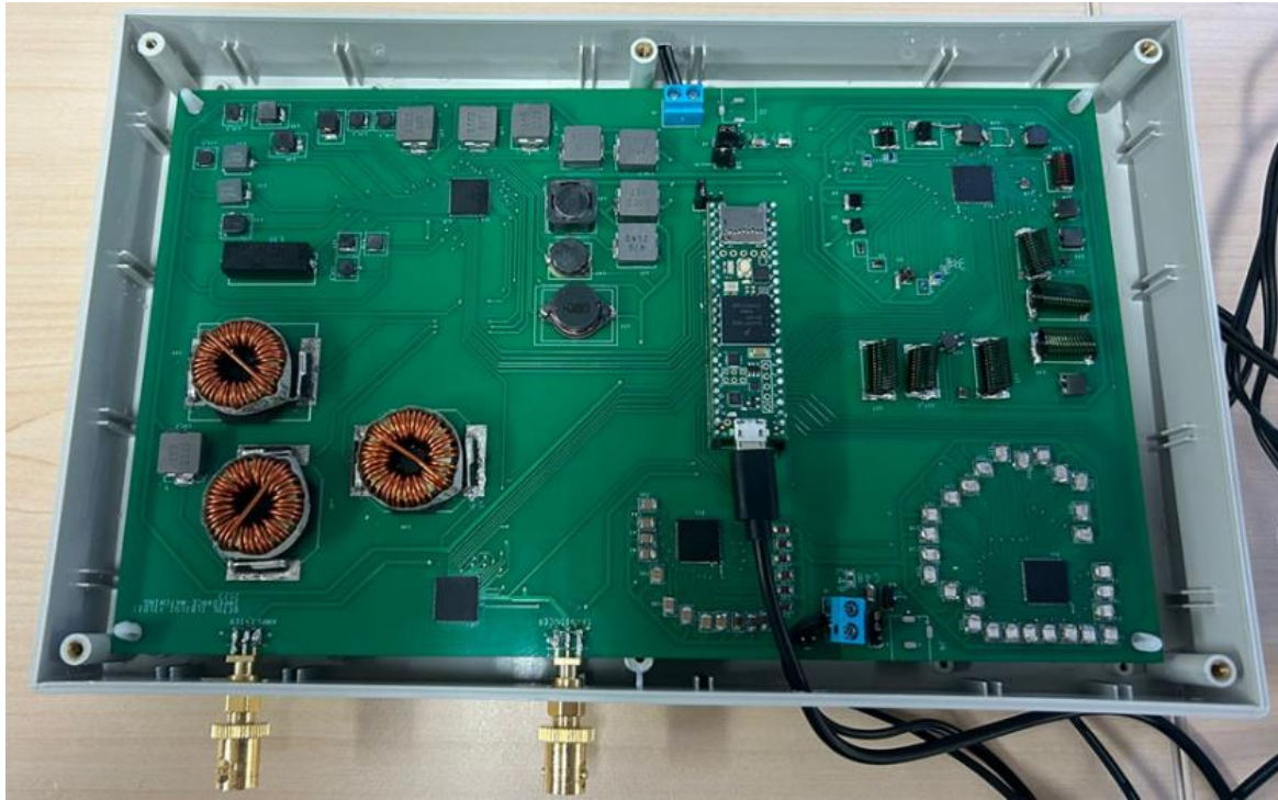
Figure 4.4. Design of a programmable matching network on a PCB.
