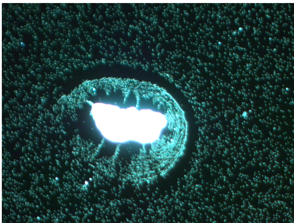
FIGURE C.7: The soft mask nano-spheres were deposited from a colloidal solution, meaning that the deposition patterns occasionally followed the flow of the liquid. Here, a dark-field microscope image shows the spheres clustering around a piece of debris – a starry night.
