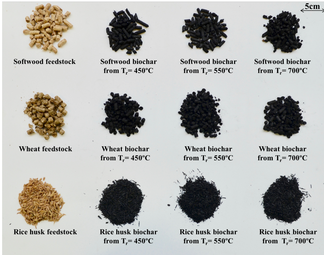
Figure 5.1: Biomass and biochar samples used, with feedstock and various biochars produced in a pyrolysis reactors at temperatures of 450 °C, 550 °C, and 700 °C for softwood, wheat, and rice husk.
