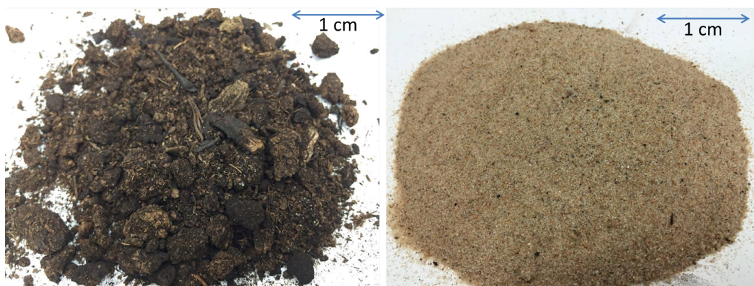
Figure 3.3: Peat (left) and sand (right) are mixed to create the appropriate inorganic content ratios of the samples.
