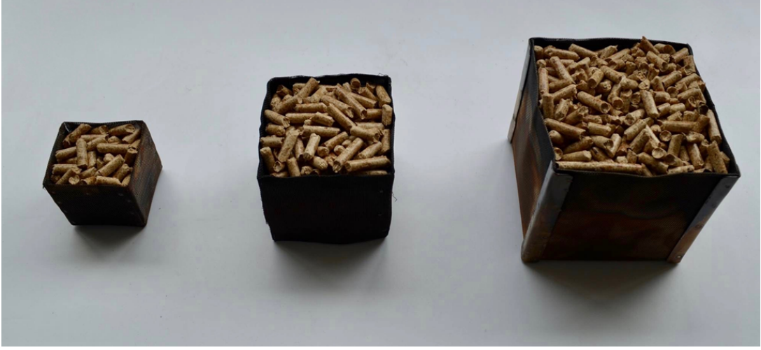
Figure 4.2: Experimental setup for studying self-heating of a biomass sample placed at the centre of the thermostatically controlled oven with thermocouples for measuring the ambient and biomass temperatures (left) and meshed experiment baskets filled with softwood feedstock (right).
