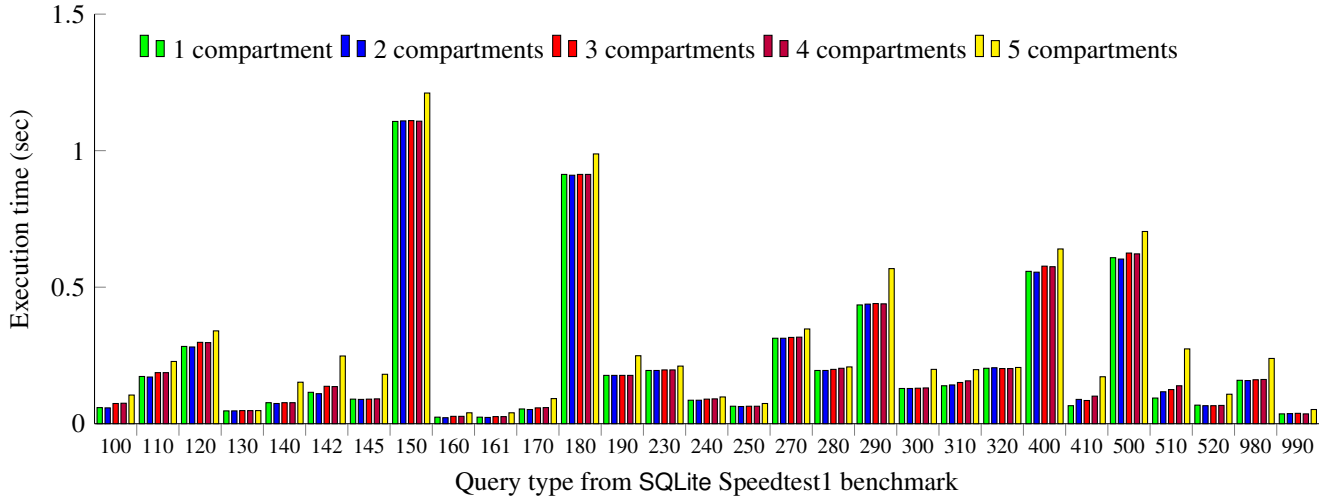
Fig. 6: Query execution times for different compartments using ORC (SQLite)
