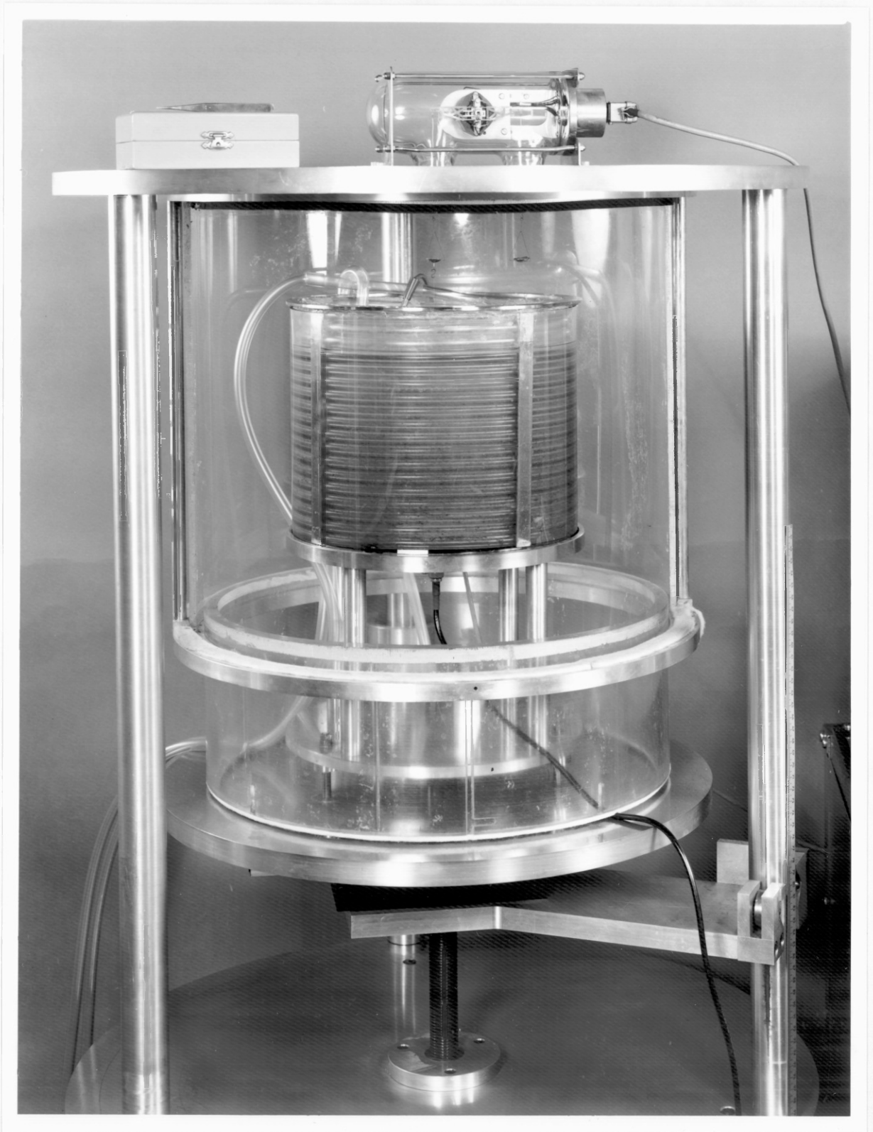
Photograph 3: The Radiation Pressure Balance.
