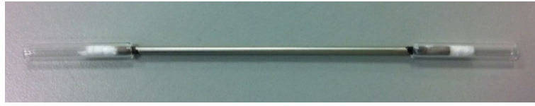
Figure 7.11: Photograph of an annealed nickel-coated YSZ hollow fibre
