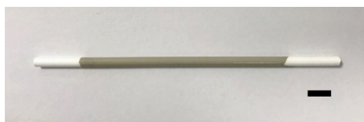
Figure 7.6: Photo of a YSZ hollow fibre after the Pd seeding step (Scale bar: 5 mm)
