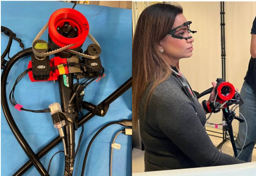
Figure 8.3 Eye Gaze steering wheel mount with thicker steering wheel and side to side mount (left) and in use (right).
