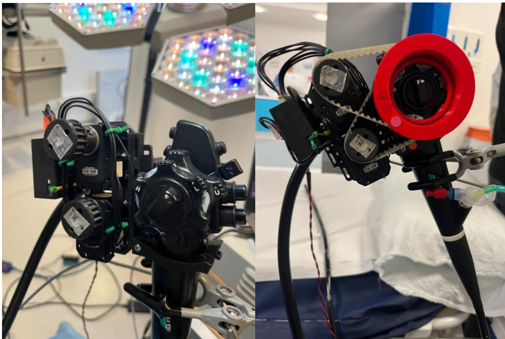
Figure 8.5 Endoscope with iGAZE2 system partially mounted for intubation (left) and with wheel and belts attached (right).
