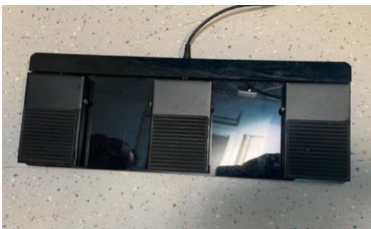
Figure 8.6 Foot pedal used to control retroflexion with two additional unmapped pedals.
