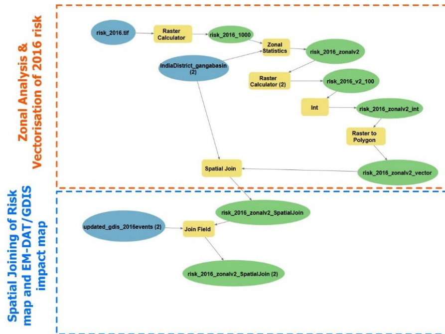
Figure 4.6: ArcGIS Model builder showing the workflow for the processing of the 2016 risk map.
