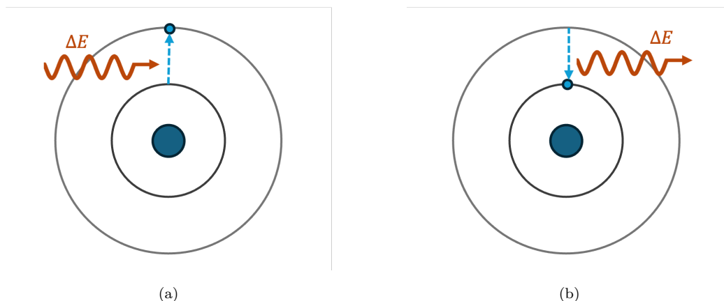
Figure. 5.3: Main light-matter forms of interaction: (a) Absorption: The atom absorbs light of energy corresponding to the difference in energy between its two states. (b) Emission: The atom emits light of energy corresponding to the difference in energy between its two states.
