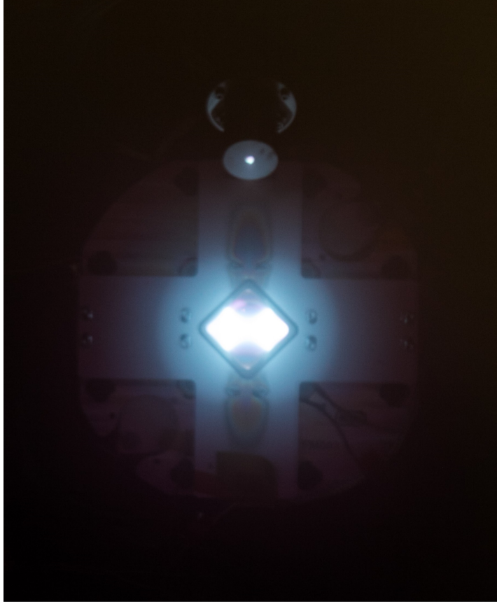
Figure 2: The discharge channel of the QCT presents peculiar light emission structures. The strongest light emission originates from two specific quadrants of the channel. The photograph shows a SSTL QCT qualification model during testing at the European Space Agency Electric Propulsion Laboratory.
