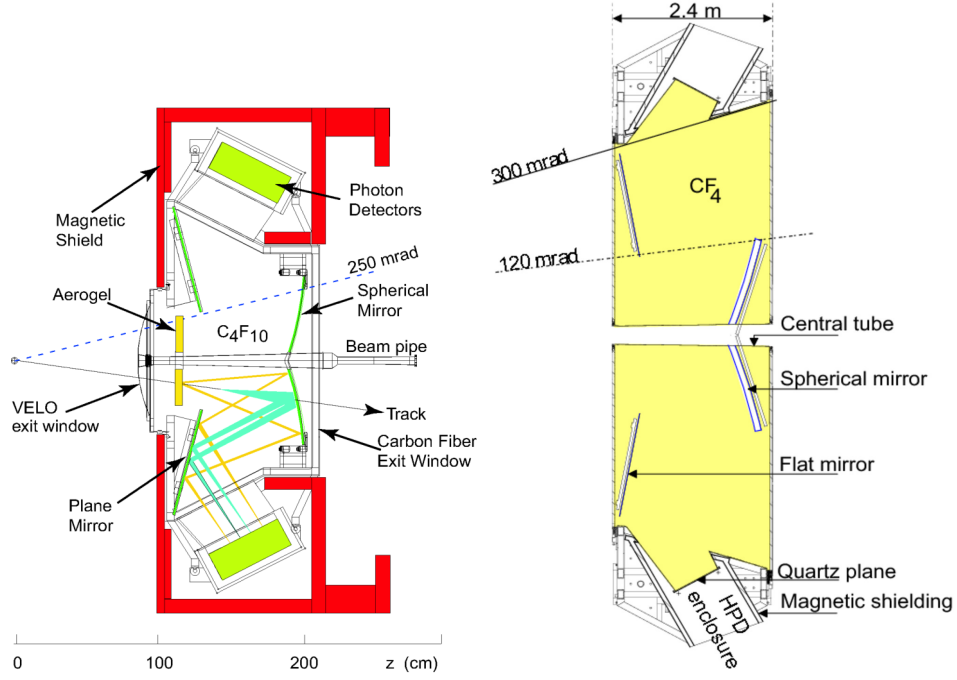
Figure 3.5: Schematic cross-sections of the (left) RICH 1 and (right) RICH 2 detectors in the y - z plane. Figure taken from Ref. [72].
