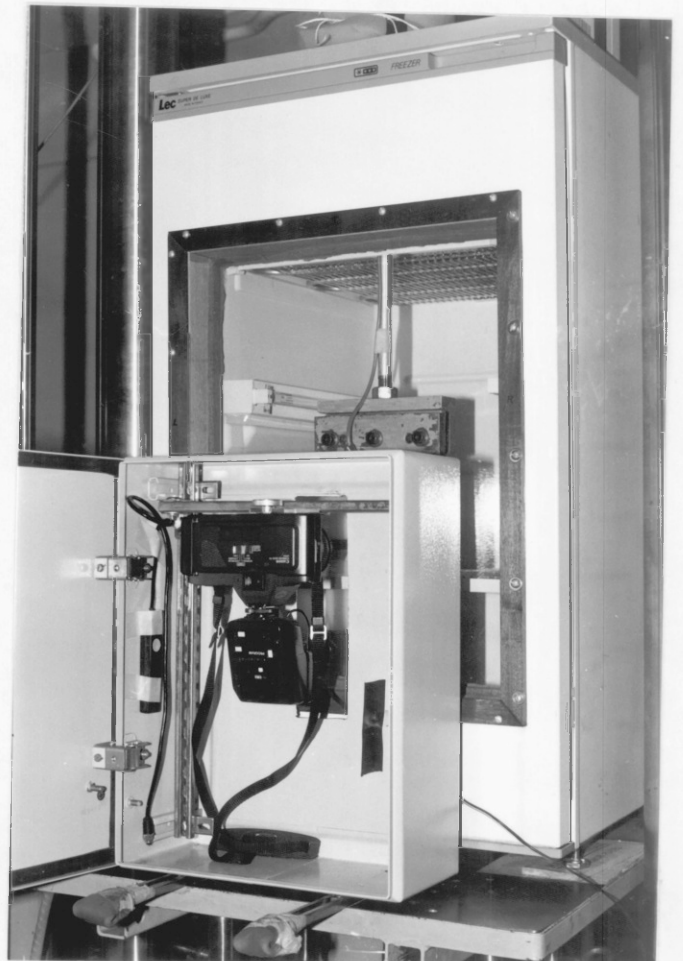
Fig 4.7 Complete testing set-up with freezer and camera used to measure crack lengths.
