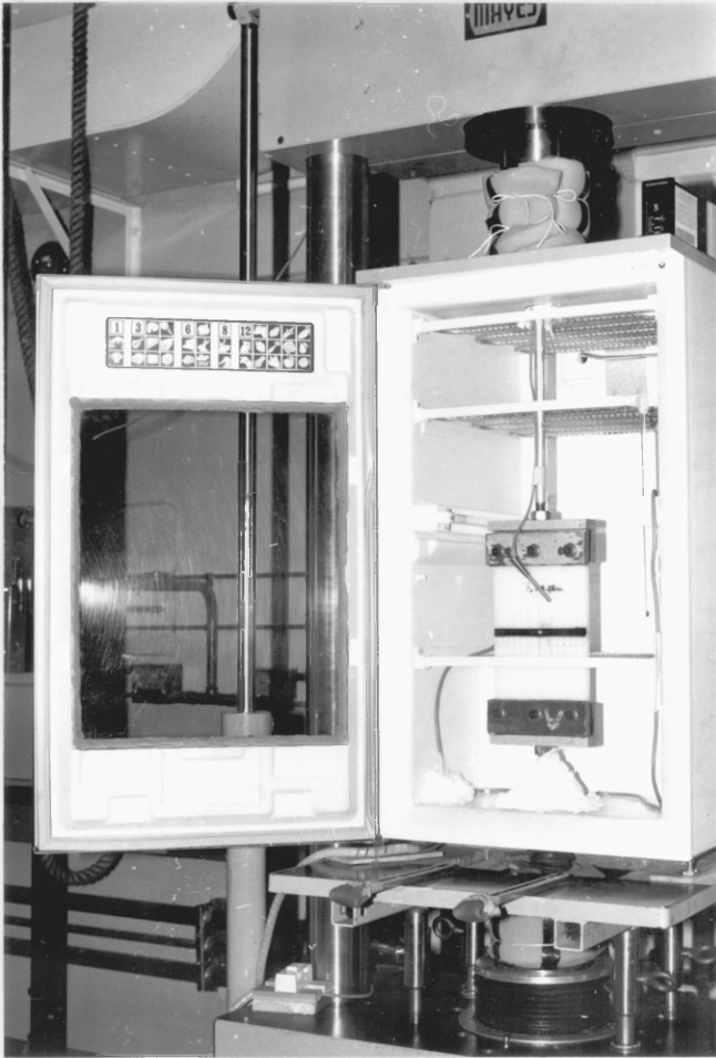
Fig 4.6 Freezer in its adapted form mounted into the Mayes servo-hydraulic machine.
