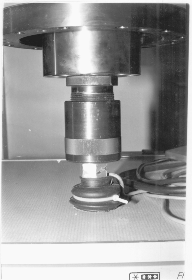
Fig 4.5 Bellows fitted so as to minimise heat loss.
