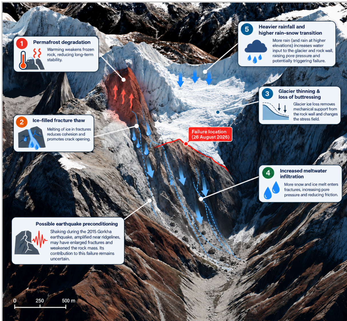
Figure 2.1: Climate-sensitive and other key preconditioning processes potentially contributing to failure. Conceptual representation of the main mechanisms through which climate variability and climate change may have influenced the stability of the Rasuwa rock wall in addition to earthquake preconditioning.
