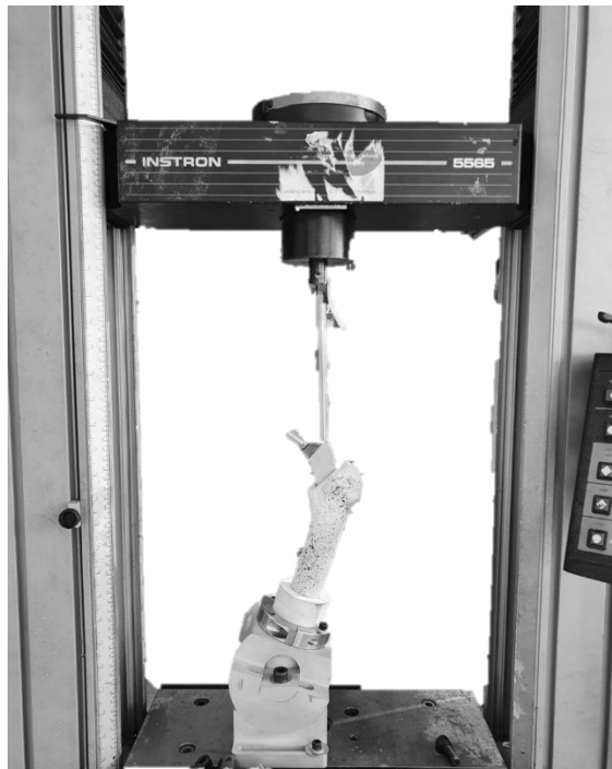
Figure 8-4 Pull-out test set-up using a uniaxial Instron
