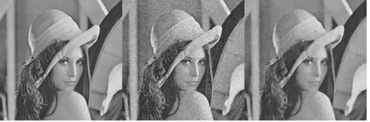
Figure 5.5: The photo on the left is the original image. The middle photo is noisy image with Gaussian noise and a standard deviation 0.05. The right image is the denoised image \mathbf{u}^* with \sigma = 3.9115 and d(\mathbf{u}^*) = 62\% . The image is the commonly used “Lena” photograph.
