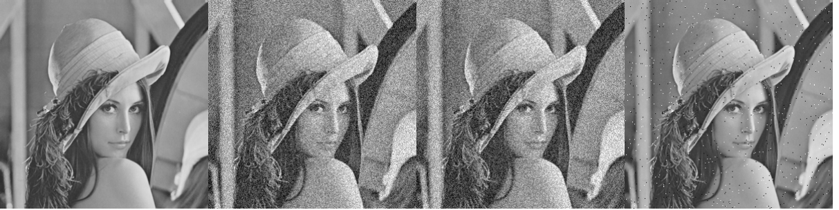
Figure 5.2: Examples of no noise, Gaussian noise, uniform noise, and salt-and-pepper noise (left to right). The standard deviation of the noise of each individual pixel is set to 0.1. The image is the commonly used “Lena” photograph.
