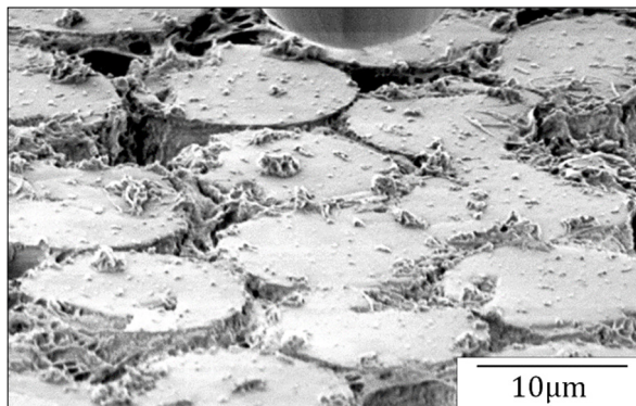
Figure 6.12 Surface of G/PP aged in pentane/toluene at 100°C for 51 days
