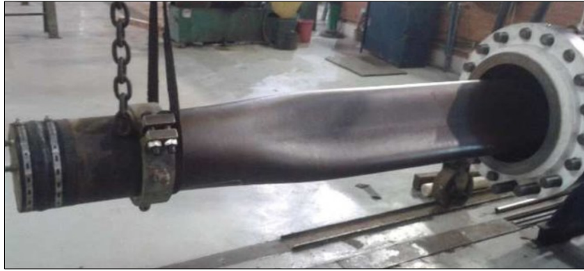
Figure 2.8 Pipe exhibiting buckle propagation after a collapse test in a hyperbaric chamber
