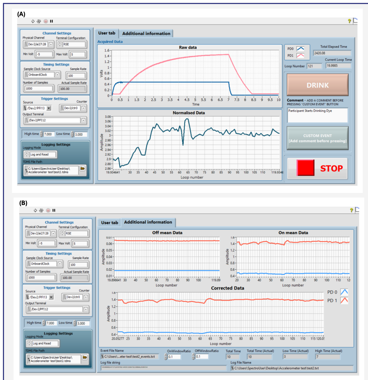
Figure 5.6: The LabView user interface developed for collection and pre-processing of data. (A) Main tab of the LabView interface showing the raw voltage data collected by the sensor photodiodes (upper graph; PD0 – Backscatter Photodiode; PD1 – Fluorescence Photodiode), the normalized fluorescence intensity data (lower graph), and the main sensor/acquisition controls. (B) Secondary interface tab with additional information (including mean 'Off' and 'On' data for each photodiode).
