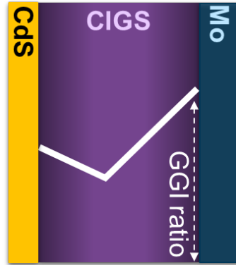
Figure 1.16: Schematic of the double Ga-gradient CIGS profile.
