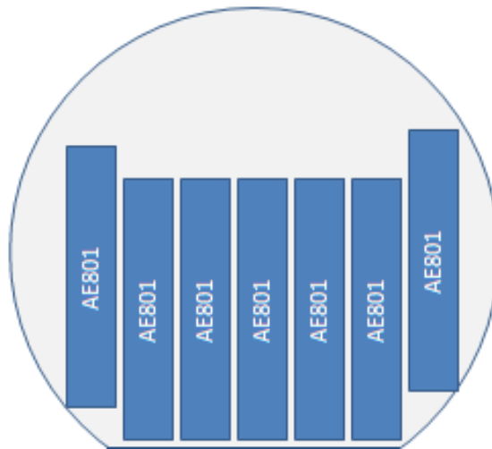
Figure A4: The orientation in which the AE801 sensing elements are profiled with respect to the “(100) silicon wafer” flat. Data and image provided with permission from Kronex Technologies Corporation (Oakland, USA) www.kronex.com .
