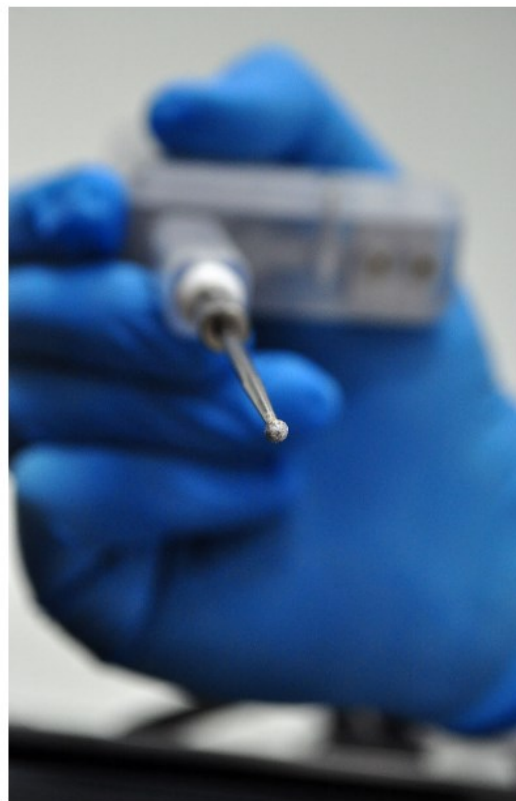
Figure 2.9 Hand-held sensory guided surgical micro-drill Brett et al ©2012 IEEE [71].
