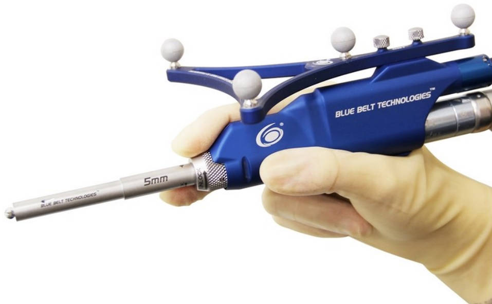
Figure 2.4 The Navio PFS TM which uses active guidance of the tool tip for resurfacing in partial knee replacement surgery courtesy of BlueBelt Technologies Inc.
