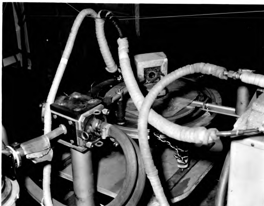
Plate General view of thermal expansion assembly and 5.1a diffractometer mounted on x-ray tube.
