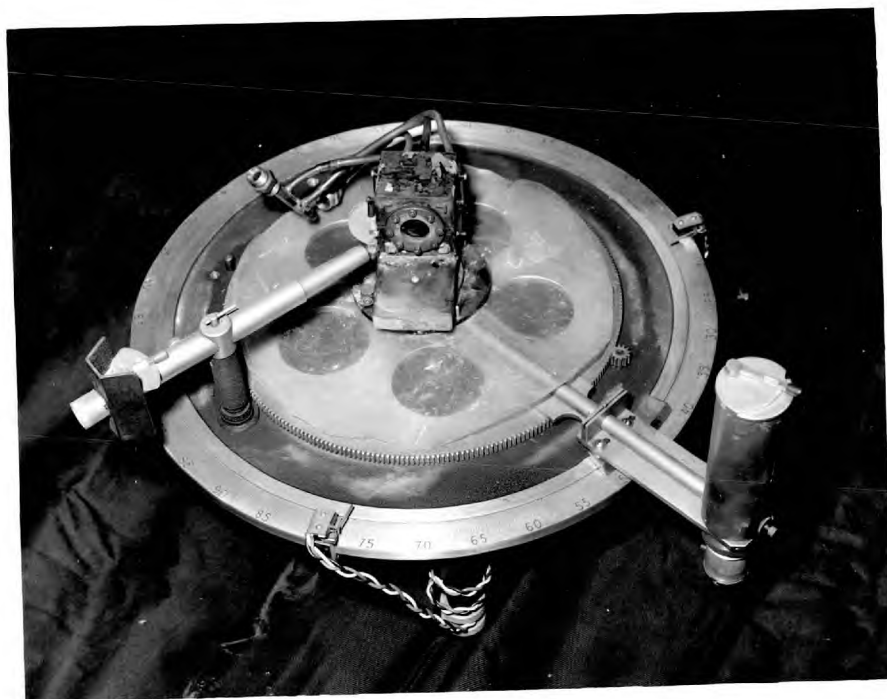
Plate Cooling block on diffractometer. The polystyrene 5.1c insulation has been removed.
