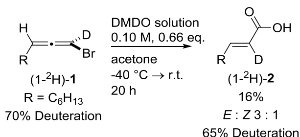
Scheme 3.2.4.1: Epoxidation of deuterium labelled (1- 2 H)-1 with DMDO solution.
