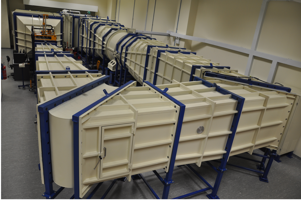
Figure 4.1: Closed-loop, sub-sonic wind tunnel at Temasek Laboratories, National University of Singapore.
