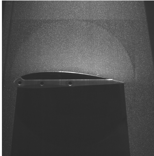
Figure 4.7: Field of view ( 225 \times 225\text{ mm} ) for PIV investigation of the whole flow around the aerofoil.
