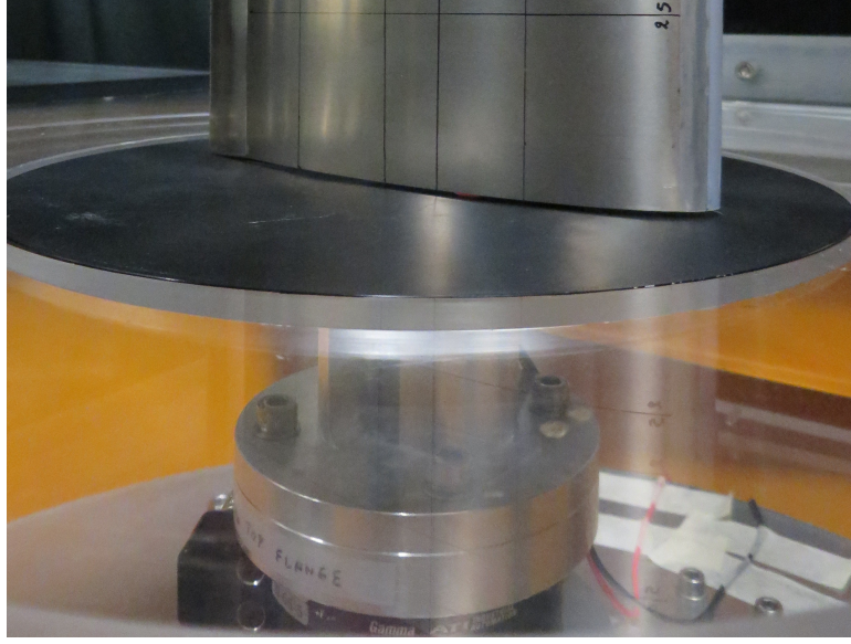
Figure 4.5: Piezoelectric gauge mounted beneath the aerofoil
