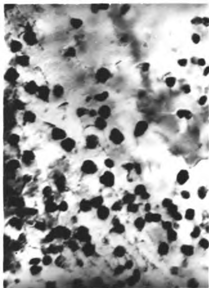
FIG 36 Solution treated aged 60 mins 700°C (x45,000)
