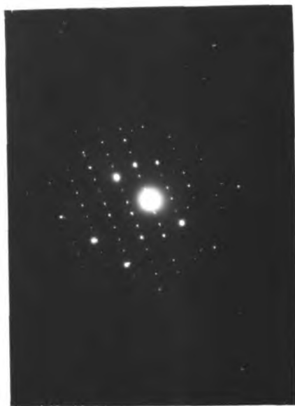
FIG 49 Solution treated aged 50,000 mins 700^{\circ}\text{C} . Selective area diffraction pattern.
