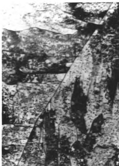
FIG 33 Solution treated aged 60 mins 600^{\circ}\text{C} (80% transformation) (x13,000)
