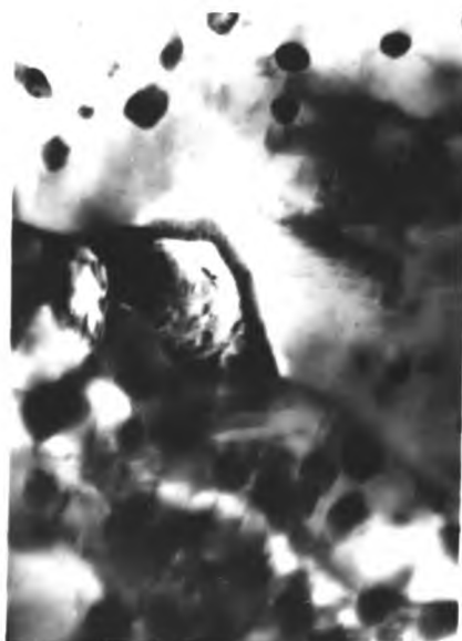
FIG 45 Solution treated, aged 1200 mins. 700°C (x45,000)
