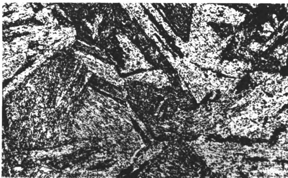
FIG.10 Solution treated 2 hrs. 1100^{\circ}\text{C} + Liq \text{N}_2 . Aged 30,000 mins. 600^{\circ}\text{C} (x350)
