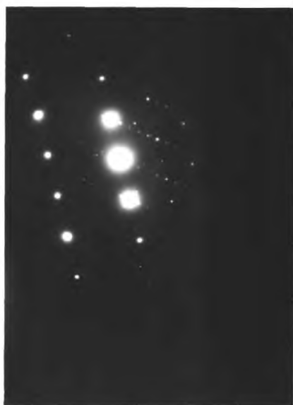
FIG 43 Selected area diffraction pattern of FIG 42
