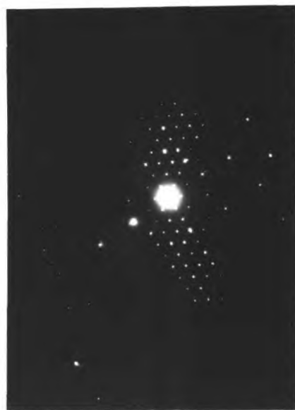
FIG 51 Solution treated aged 50,000 mins 700^{\circ}\text{C} . Selective area diffraction pattern.
