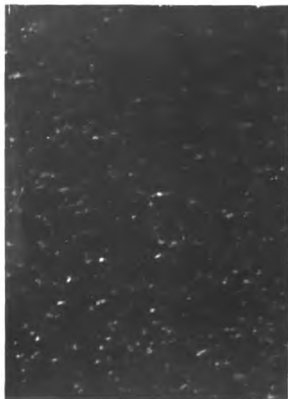
Fig 26 Dark field micrograph of specimen solution treated, aged 40 mins 600^{\circ}\text{C} (65% transformation) (x45,000)
