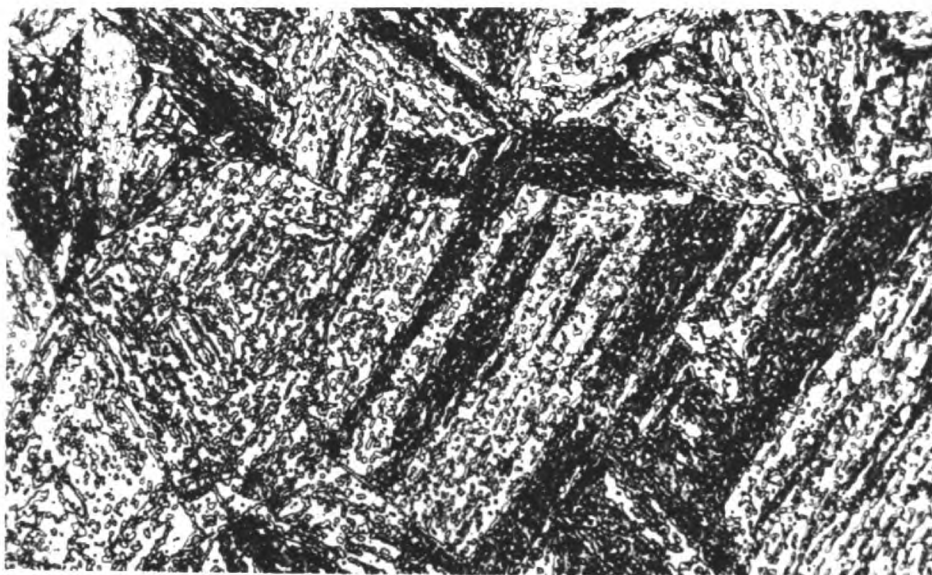
FIG 12 Solution treated 2 hrs: 1100^{\circ}\text{C} + Liq \text{N}_2 Aged 30,000 mins. 700^{\circ}\text{C} . (x350)
