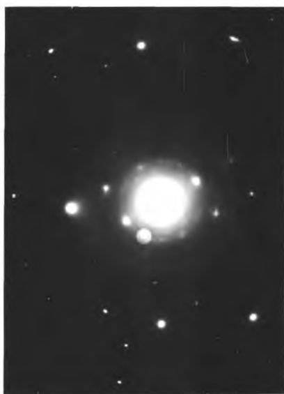
FIG 23 Selected area diffraction pattern of Fig 21.
