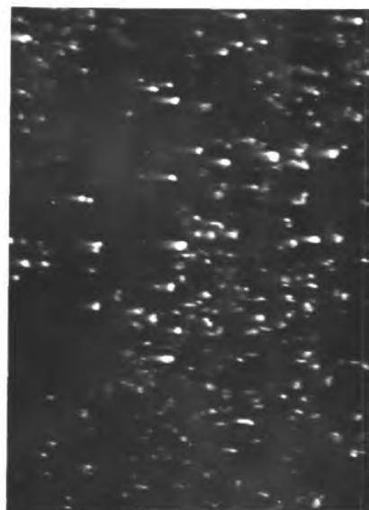
FIG 30 Dark field micrograph of FIG 29 using precipitate reflection (x45,000).
