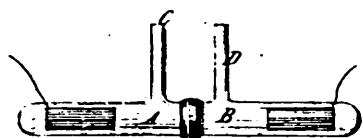
Figure 3.7 Streaming potential apparatus of Quinke (1859) (explanation of figure in text)
