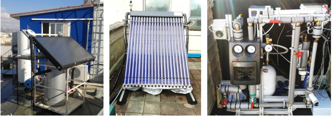
Fig. 3. Test setup: a) Solar collector testing apparatus with storage tank in Limassol used for testing of FPC and PVT collector (shown); b) ETC collector; and c) control apparatus including pump, electric heater, flow meter and temperature controller used in the London testing apparatus
