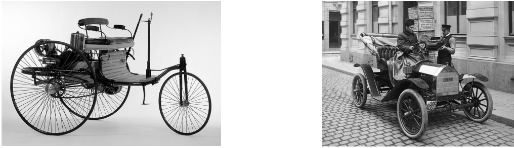
Fig. 2.1: Benz Patent-Motorwagen (left), a two-seater, three-wheeled vehicle built in 1886, is regarded as the first automobile. Its suspension comprised elliptic springs in the rear axle. In 1906, the Brush Two-Seatby Runabout (right) was the first car equipped with coild springs and shock absorbers. Photographs from [Daimler AG, 2015a; Wikipedia, 2015a].
