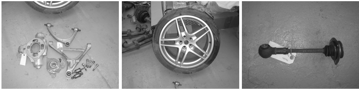
Fig. 7.8: Top and lower wishbones, bushings, wheel bearing, hub carrier and wheel bolts (left), rim and tyre (centre) and tie rod (right).
