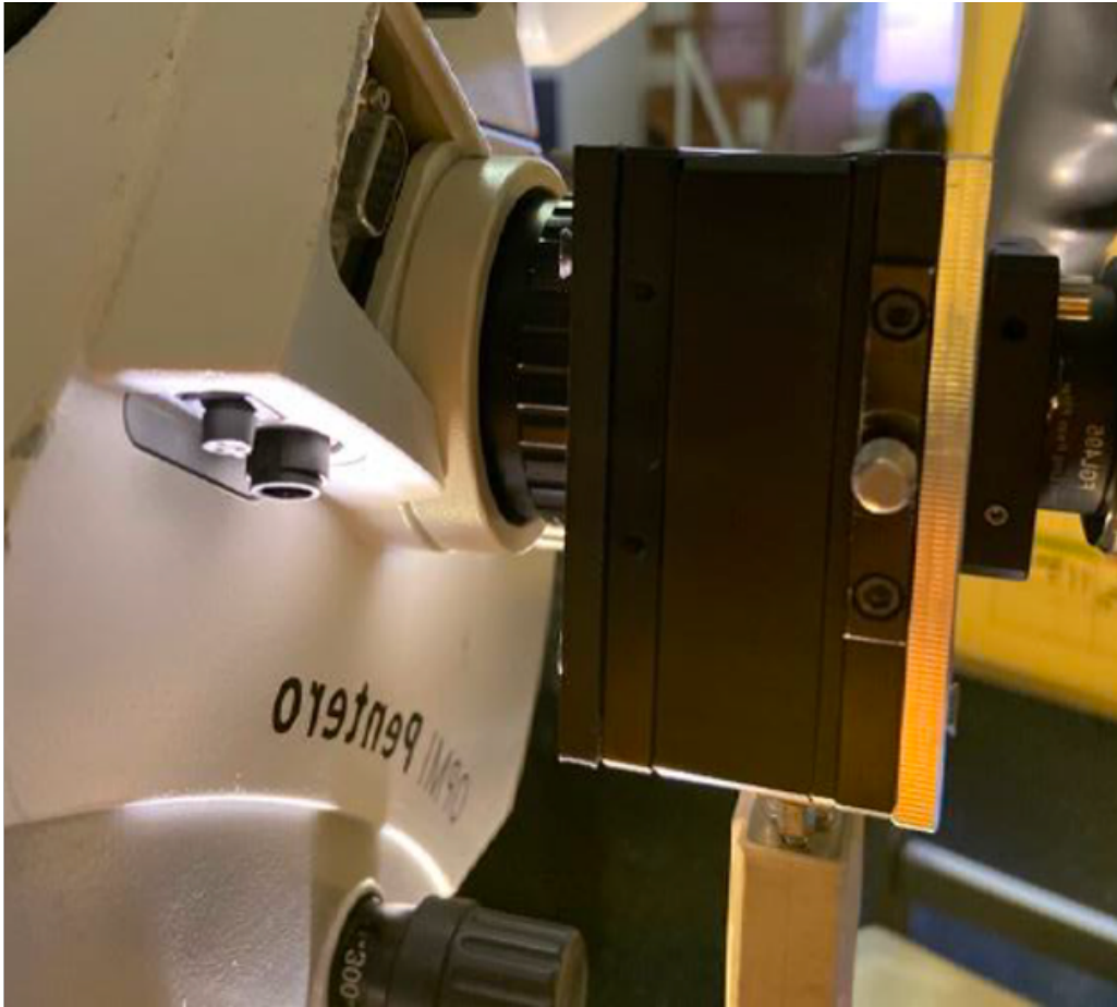
Figure 4.5: Adapter connecting the Pentero port with the LCTF and the camera
