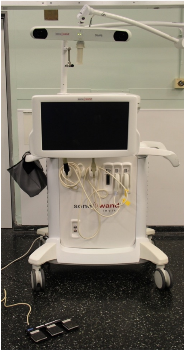
(a) Main device: screen, main bulk with probes (bottom centre), pedals (bottom left), infrared camera (top centre)
