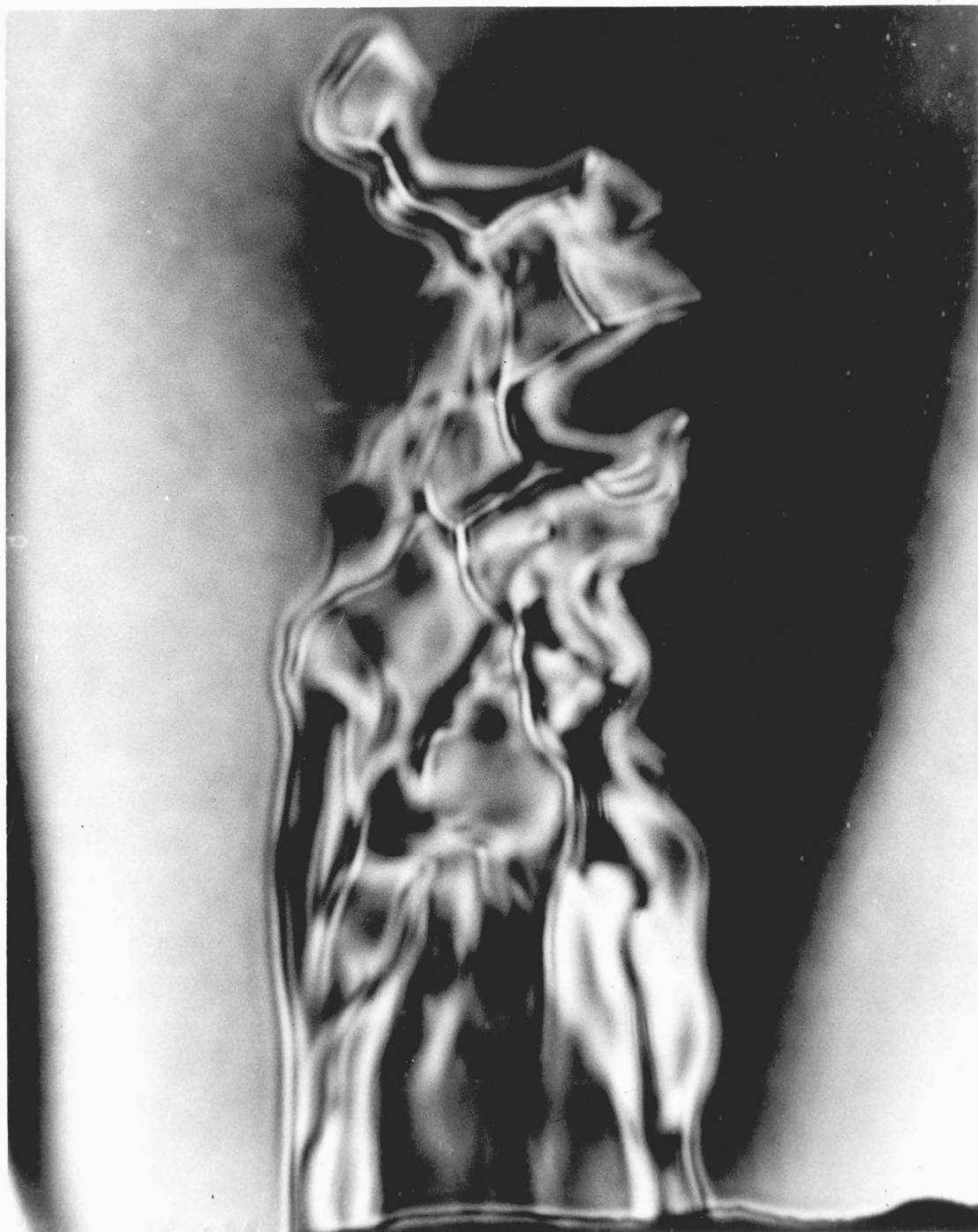
FIGURE 8 - INSTANTANEOUS SCHLIEREN CONTOUR OF TURBULENT FLAME
