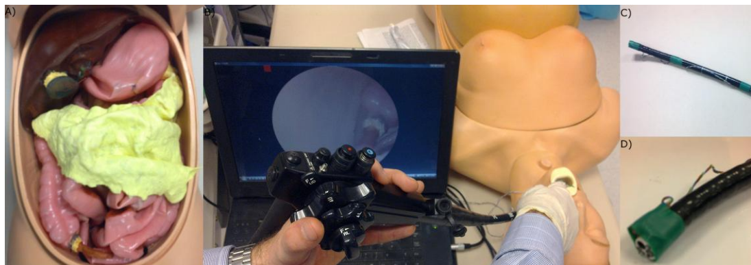
Figure 7.1 a) Overview of the abdominal components of the ELITE simulator with gastrostomy site visibly marked by sutures b) Experimental set-up with unaltered endoscopic view c&d) Flexible endoscope with IMU mounted at tip
