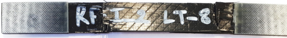
Figure 4.6: Failed tension specimen.
