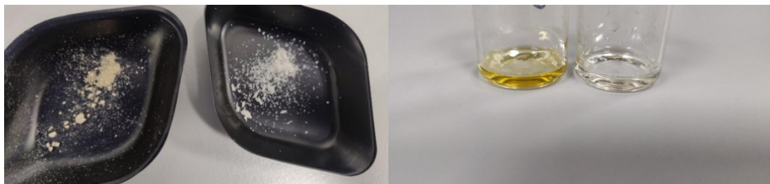
Figure A. 23 Comparison between the commercial DFF and the sublimed material (left) and comparison of the bulk IL after first sublimation and second sublimation (right).
