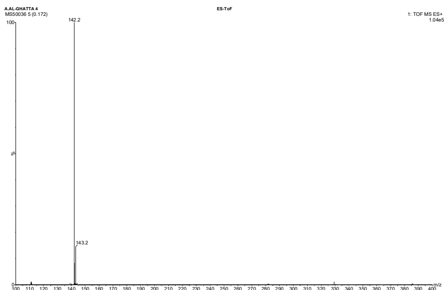
Figure A. 11 Mass spectrum of [bmpyr]OTf.
