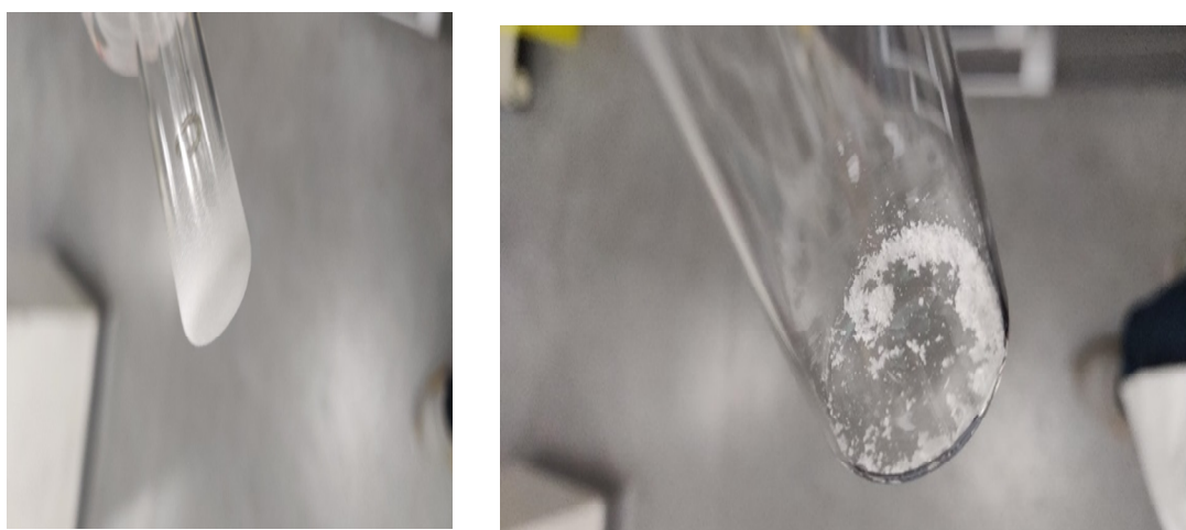
Figure A. 22 Sublimed DFF from the IL on the condenser tip (left) and collected DFF (right).
