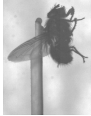
Figure 4.3: Blowfly attached to a wooden holder using a mixture of beeswax and Collophonium.
