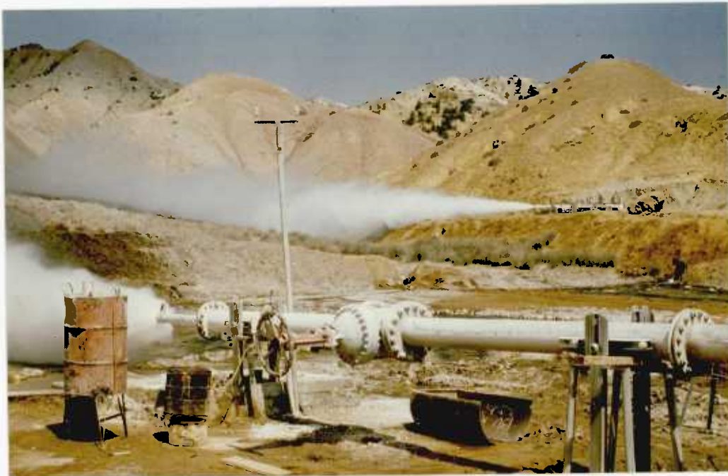
Fig. 1.12. Natural boron-containing steam wells at Saraykoy Denizli.
