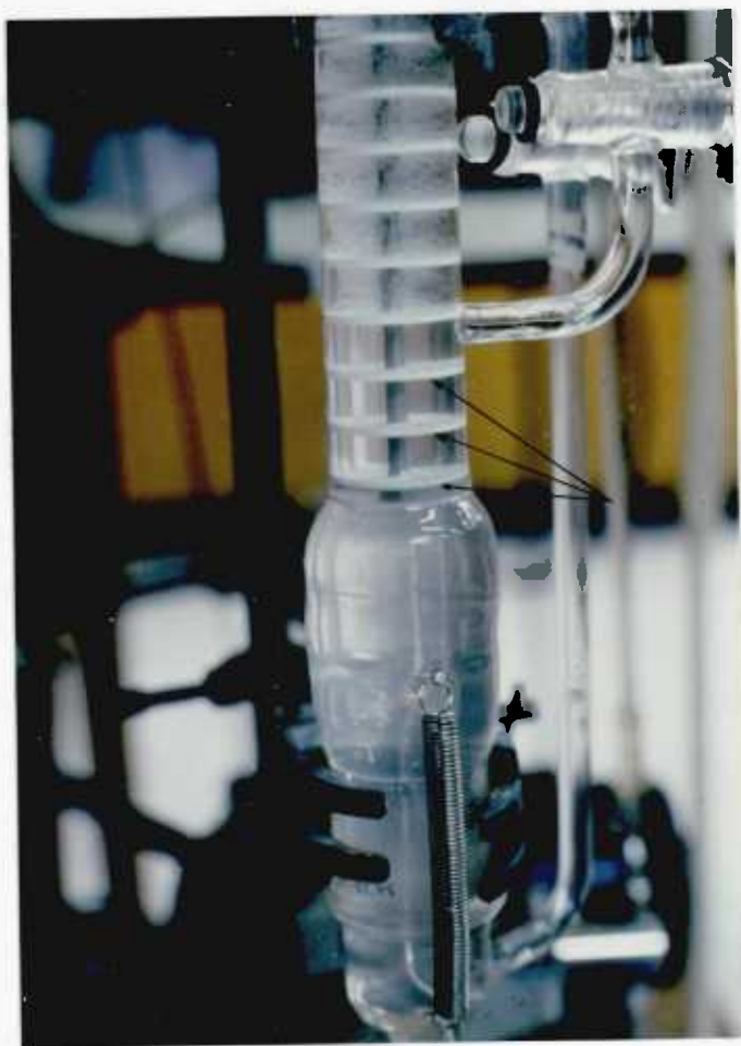
Fig. 4.15 Photograph showing the operation of the column under modified conditions (the arrows show the position of the 7 mm holes).
