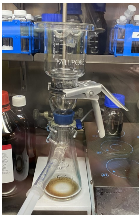
Figure 5.1 Manual vacuum filtration set-up.
