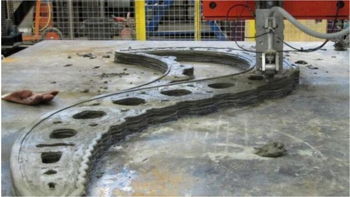
Figure 2.11: A test structure being formed through concrete printing (BBC News, 2016).
