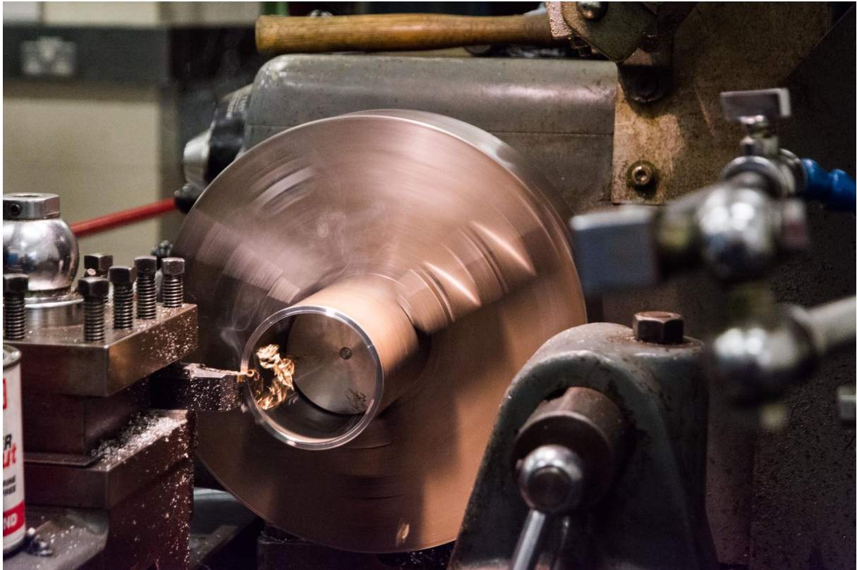
Figure 3.6: A short CHS specimen being machined, with the aluminium insert visible.
