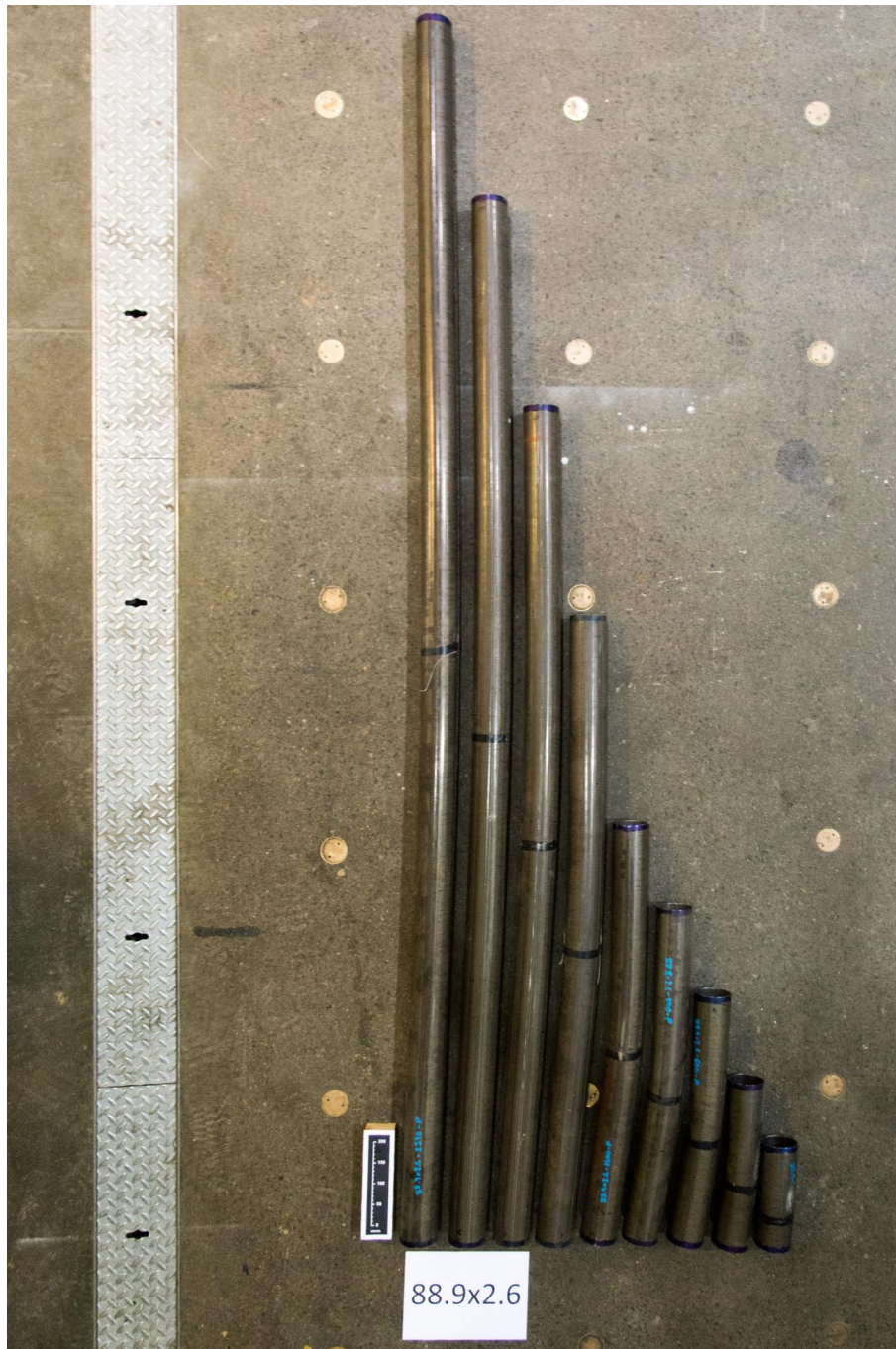
Figure 4.10: The deformed duplex 88.9×2.6 CHS long columns.
