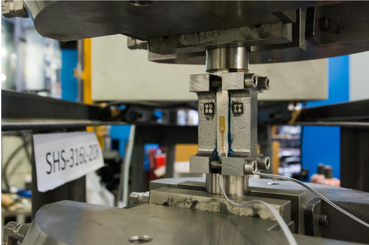
Figure 6.21: The compression coupon test setup.
