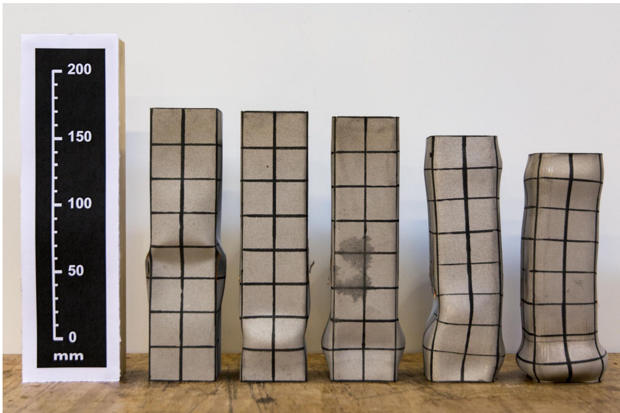
Figure 6.30: The deformed 50×50×1, 50×50×2, 50×50×3, 50×50×4 and 50×50×5 SHS stub columns, from left to right.
