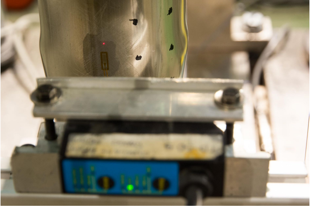
Figure 4.4: The laser distance measurement sensor at UPC.
