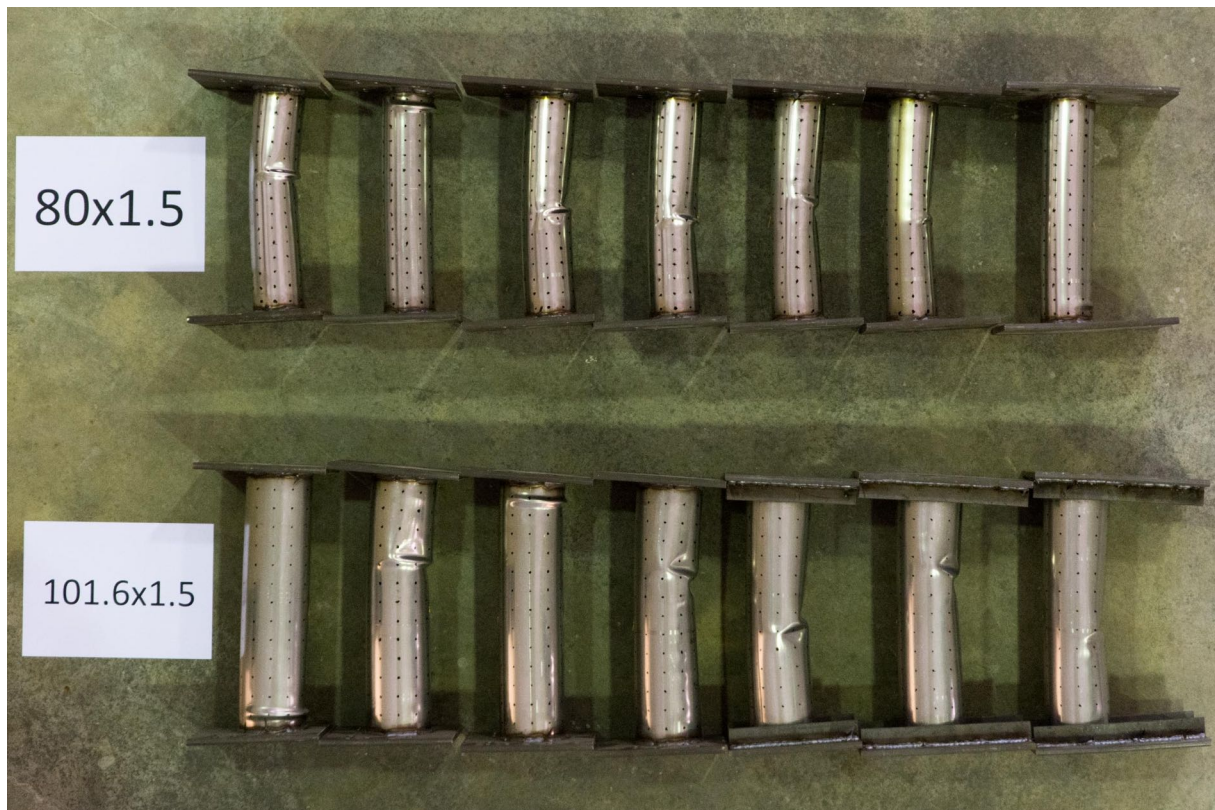
Figure 5.5: The deformed short beam-columns, with load eccentricity increasing from left to right.
