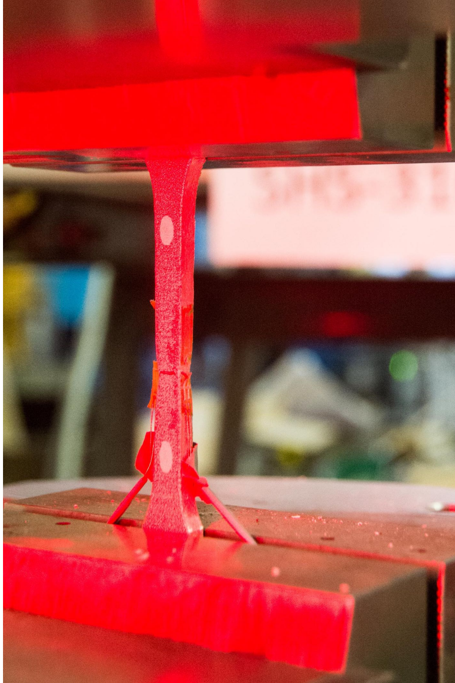
Figure 6.9: A fractured 316L tensile coupon at the end of a test.
