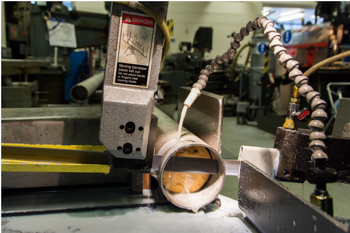
Figure 3.5: A CHS specimen being cut using a bandsaw, with wooden inserts inside and outside the specimen.
