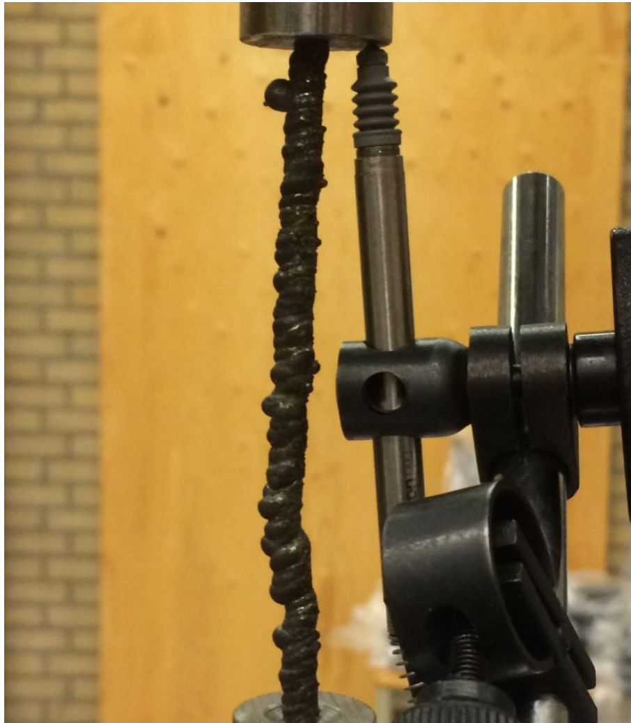
Figure 2.13: An MX3D flexural buckling test specimen (Joosten, 2015).
