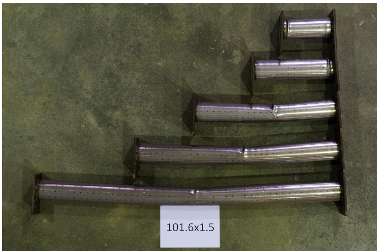
Figure 4.12: The deformed ferritic 101.6 \times 1.5 CHS long columns.
