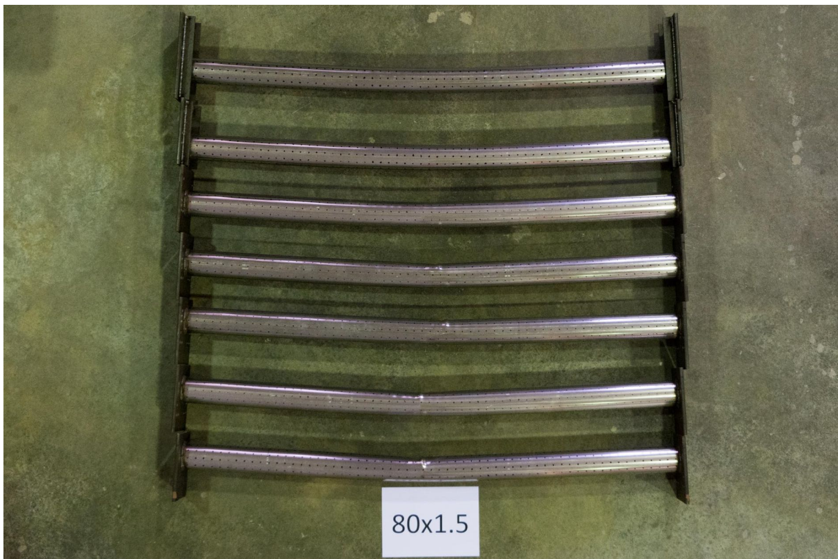
Figure 5.10: The deformed 80×1.5 CHS long beam-columns, with load eccentricity increasing from bottom to top.
