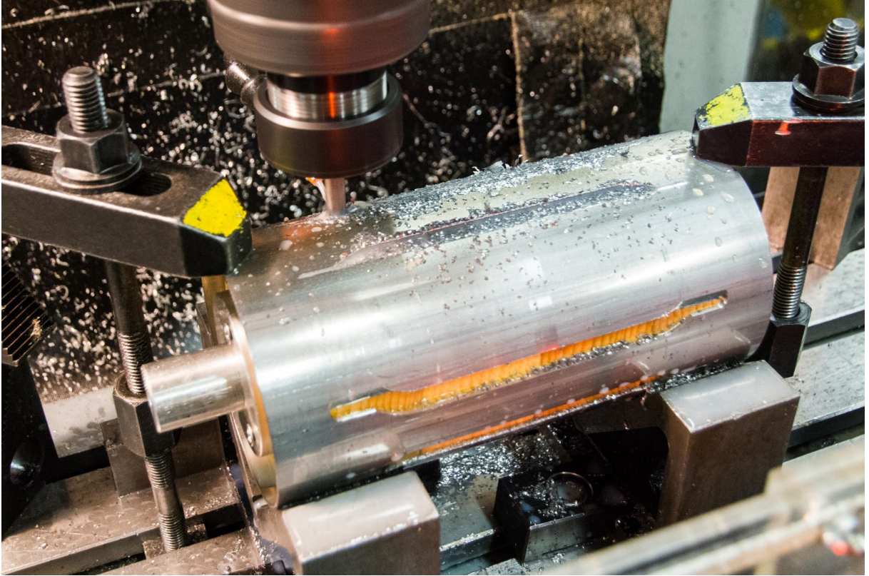
Figure 3.8: A CHS coupon being machined, with the wooden block visible.
