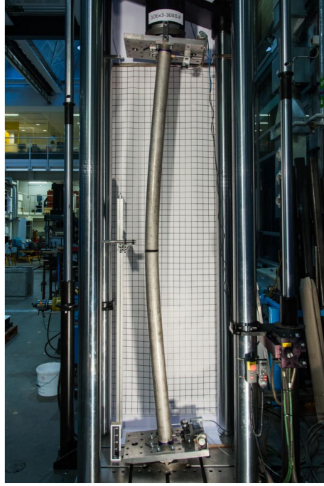
Figure 4.18: Experimental and FE failure modes for the 106×3-3080-P CHS specimen.
