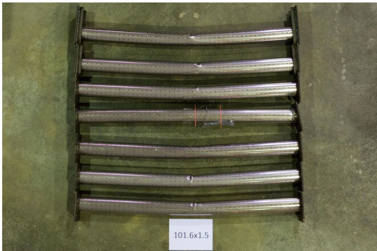
Figure 5.11: The deformed 101.6×1.5 CHS long beam-columns, with load eccentricity increasing from bottom to top, including the unsuccessful test specimens.
