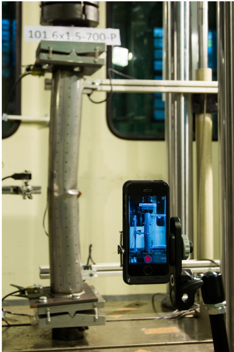
Figure 4.5: A flexural buckling test being filmed for later review.
