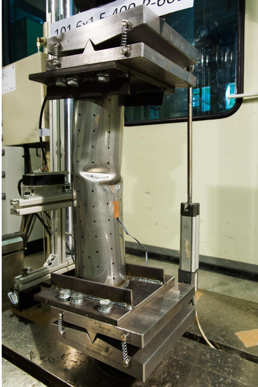
Figure 5.7: The deformed short beam-column with welded stiffeners on the end plates.
