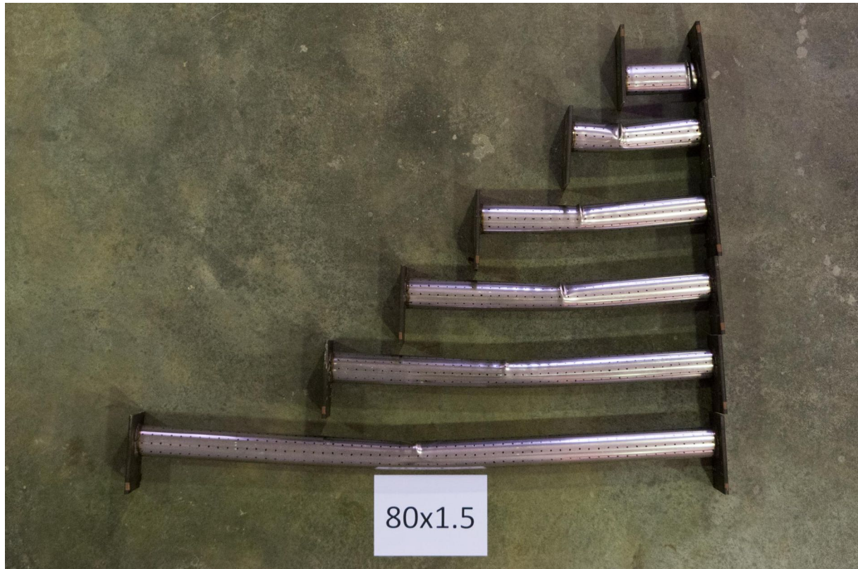
Figure 4.11: The deformed ferritic 80 \times 1.5 CHS long columns.
