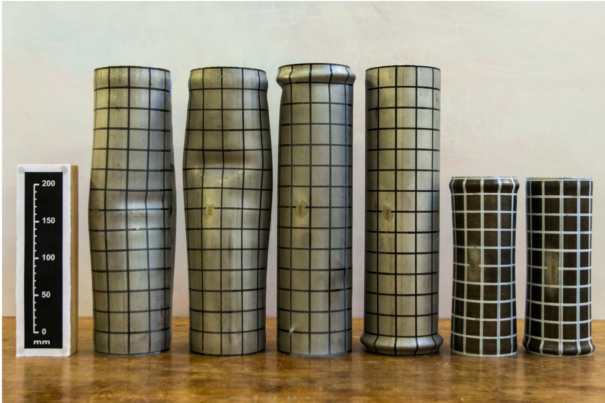
Figure 3.17: The deformed 106×3-400-F, 106×3-400-FR, 104×2-400-F, 104×2-400-FR, 88.9×2.6-250-F and 88.9×2.6-250-FR CHS stub columns, from left to right.
