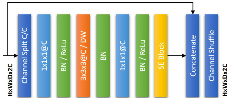
Figure 6.2: Integration of a Squeeze - and - Excitation block [Hu et al., 2018] inside a Shufflenet v2 basic block
