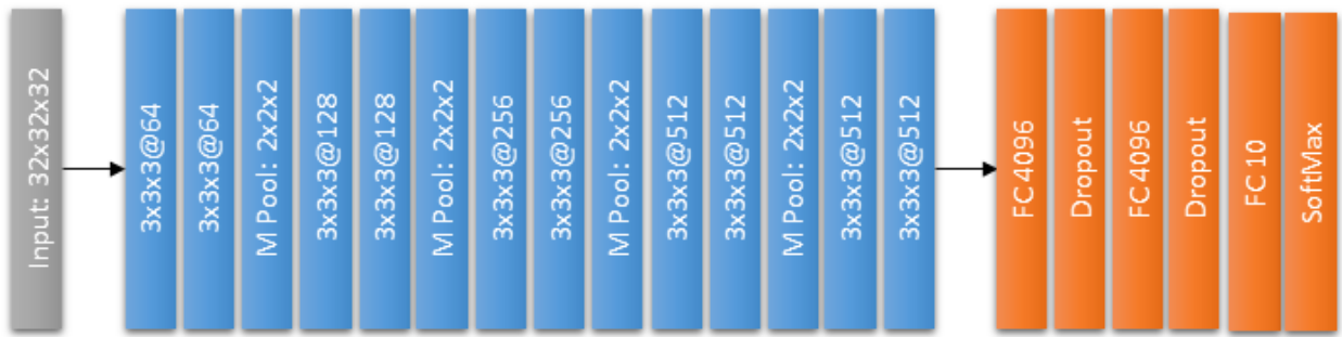
Figure 6.6: The baseline VGG13 3D architecture. It takes as input a 32 \times 32 \times 32 voxel grid, and predicts the label of the object depicted in the voxel grid
