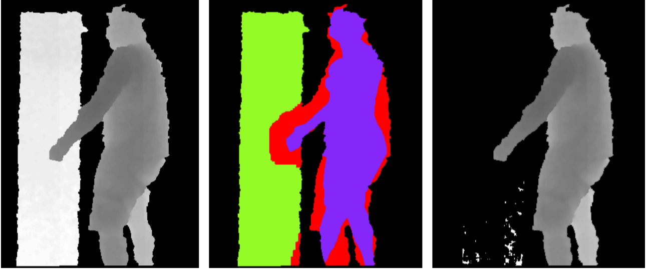
Figure 4.7: Data preprocessing for large object removal. The input image is split in three regions: blue - overlap with the last tracked human silhouette, red - buffer zone, green - candidate large object area which provides the seeds for the flood-fill algorithm. The image on the right is the processed image passed to the optimiser
