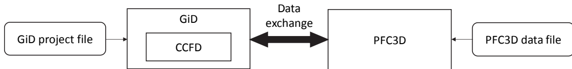
Figure 4.5 Process of conducting DEM-CFD program
