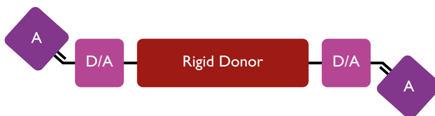
Figure 5.102 – Schematic illustrating a calamitic NFA with a rigid donor core and flanking acceptor units 38
