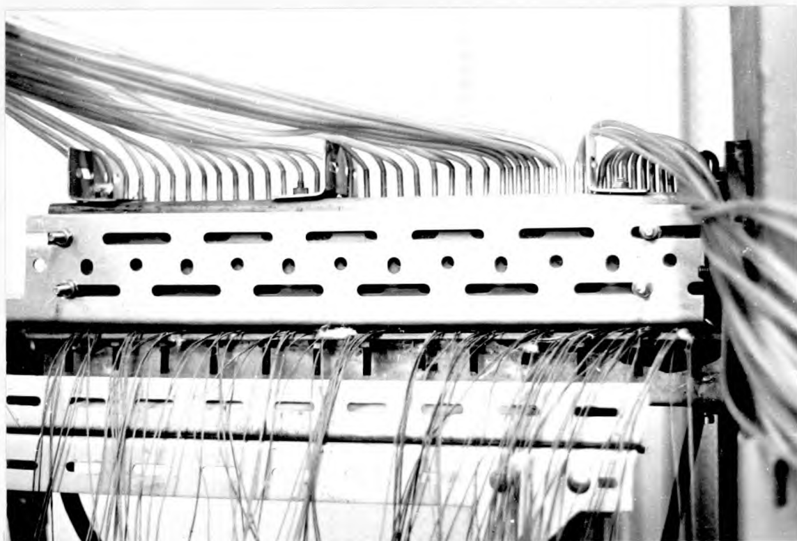
Fig. 4.5. Photograph of Tufnol Diffuser - Ejector with static pressure connections, thermocouples from heat flux meters and the underslung water jacket.
