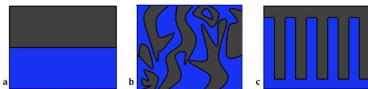
Figure 1.10 – Morphological pictures of the active layer structure for a) a bilayer b) a random two pure phase BHJ commonly used to describe the blend in many OPV devices, and c) a potential rigid network structure with a controlled and well defined phase segregation.
