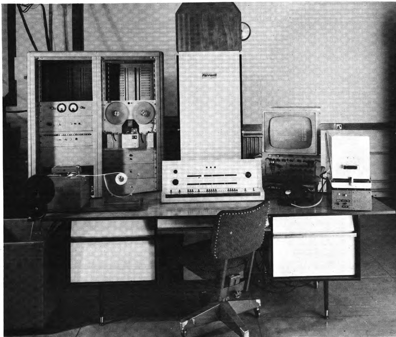
Ferranti 'Hermes' computer with visual display unit showing logged data.
