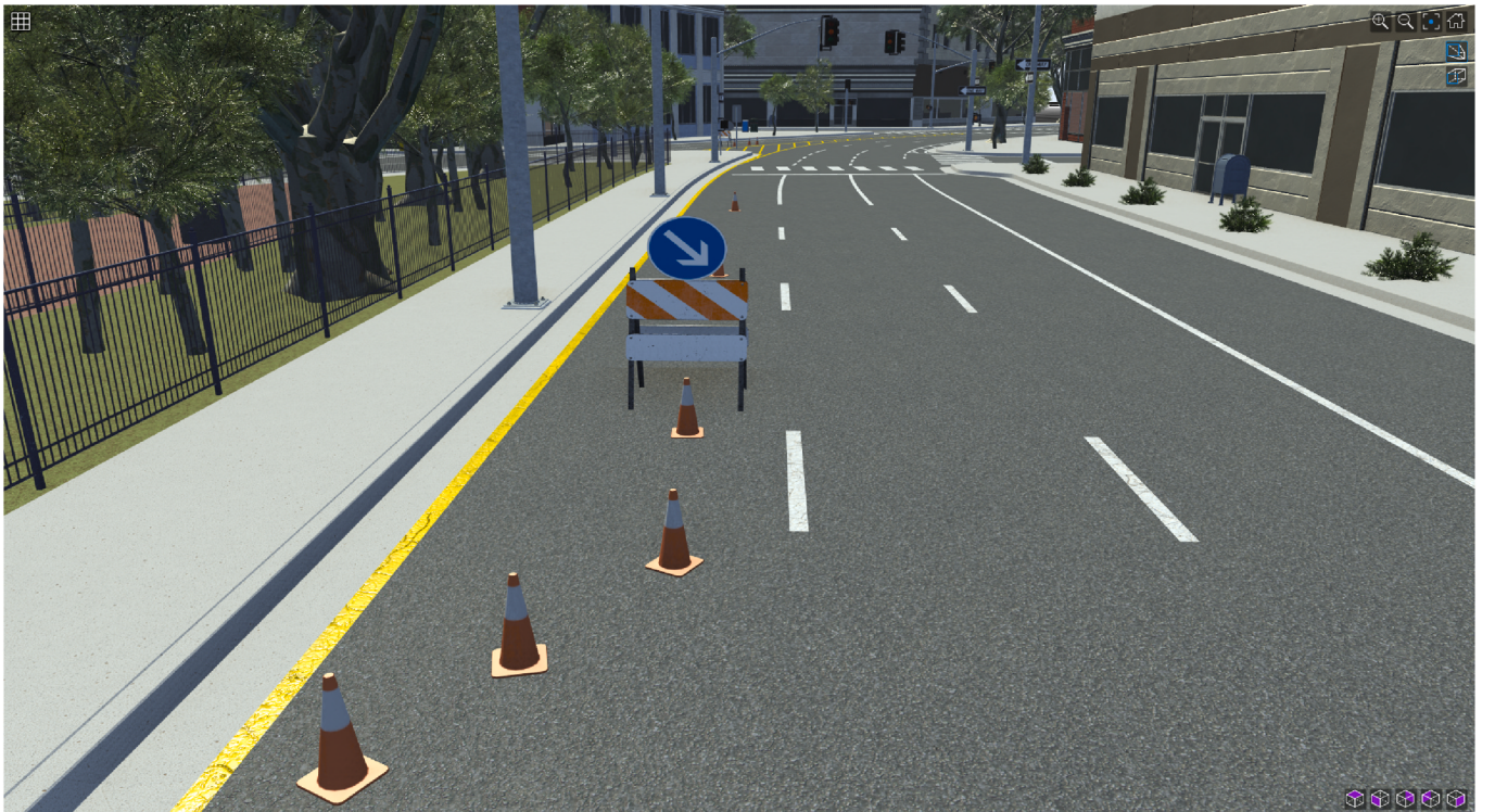
Fig. 7. Driving scenarios containing roadworks generated by RoadRunner.
