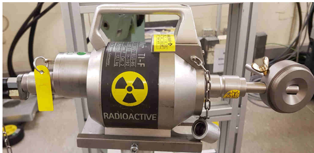
Figure 2.3 Photo of a portable transport container of a \gamma -ray source (a radiation tip and a collimator are mounted on the right of the container in order to control the spatial exposure intensity)
