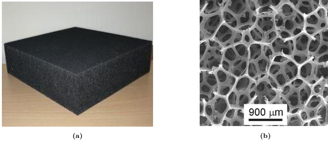
Figure 4.1: (a): 40 pores per inch (ppi) Acoustaf foam reticulated foam used in this research [153]. (b): Scanning electron micrograph of 40 ppi polyurethane open-cell foam (Hitachi S-3500-N, 10 kV accelerating voltage) exhibiting the high void fraction relative to the skeletal mass [154].
