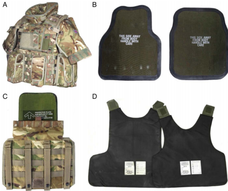
Figure 4.8: Mark 4a OSPREY armor system (A) carrier made of Cordura® 1000D nylon fabric. This system includes (B) contoured hard front and rear ballistic plates, (C) side ballistic plates and (D) filler soft armour designed to prevent fragmentation impact injuries. Reproduced from [14].
