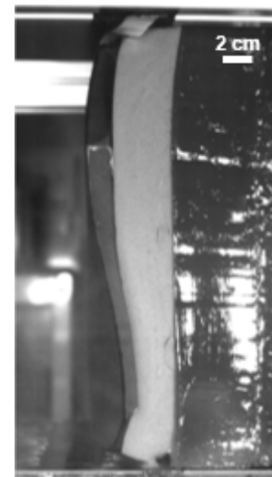
(f) Ballistic plate (backed with a 40 mm length of 20 ppi reticulated polyurethane foam).
