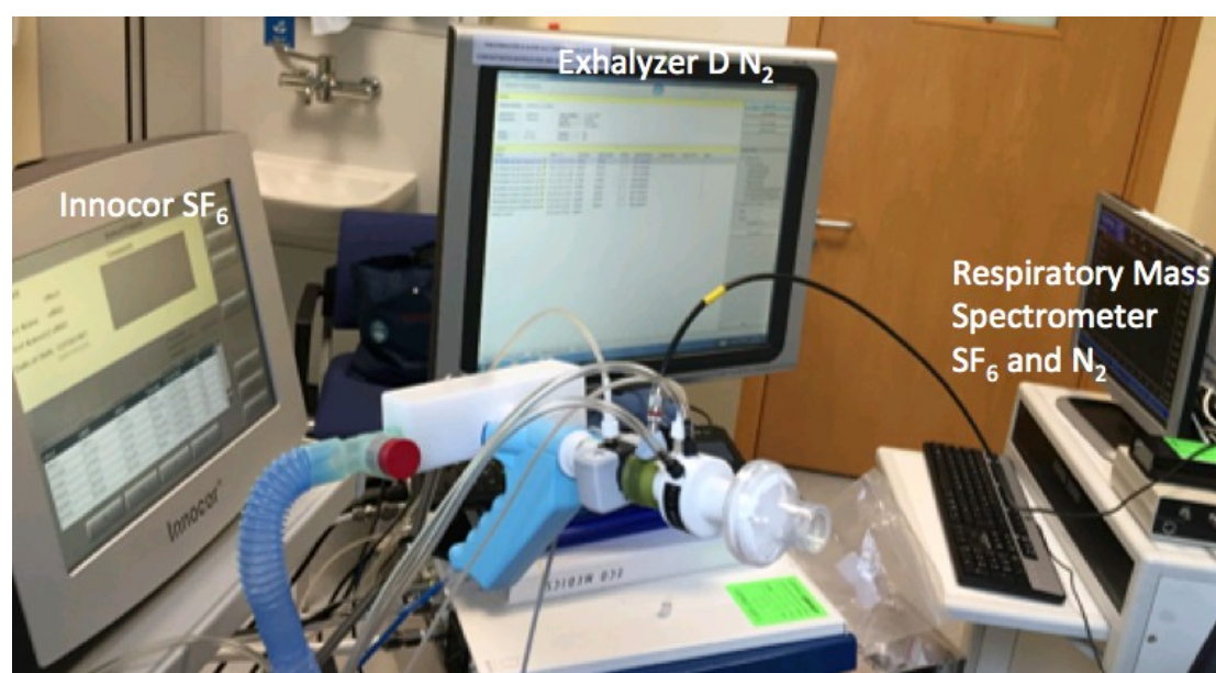
Figure 2.9 The set up of simultaneous gas washout using the modified Innocor device, the Exhalyzer D and the respiratory mass spectrometer. The flowmeters were attached together and mounted so that the patient could complete a multiple breath washout of both SF 6 and N 2 using 100% O 2 as a washout gas.
